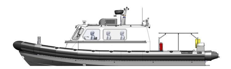
Fully enclosed wheelhouse variant of the well proven and hugely successful 1200 Fast Raiding, Interception & Special Forces Craft (FRISC®) offering comfortable shock mitigation crew seating for up to eight (8) persons or six (6) plus a stretcher case in an air conditioned wheelhouse environment with optional welfare facilities, ballistic protection and speeds up to 48 knots.
